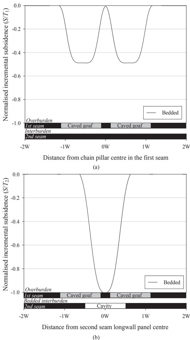
Fig. 10. Plots of incremental subsidence profiles from the staggered arrangement after extraction of the longwall in (a) the first seam and (b) the second seam.
