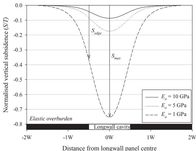
Fig. 3. Subsidence normalised by extracted seam height for an elastic overburden material with varying Young's modulus of the strata ( $E_o$ ) – Cavity Model.
