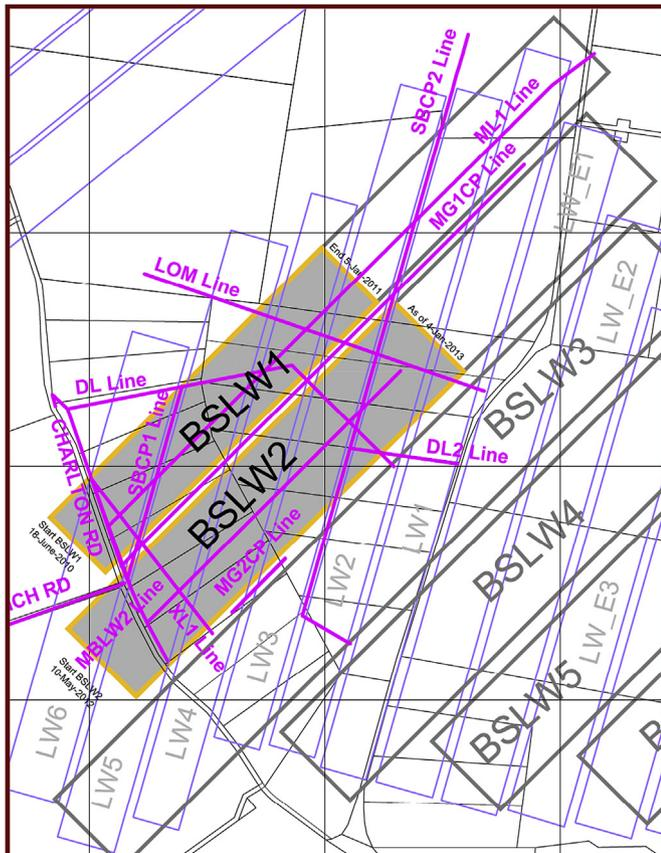
Fig. 11. Map showing the survey lines used to monitor the subsidence when extracting longwall BSLW2 (MSEC, 2013).
