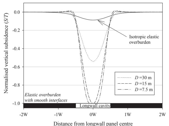
Fig. 7. Normalised surface subsidence for an elastic overburden material containing smooth horizontal interfaces separated by spacing  $D$  – Cavity Model.
