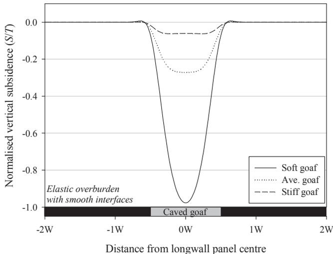
Fig. 8. Normalised surface subsidence for an elastic overburden material containing smooth horizontal interfaces spaced every 7.5 m – Goaf Model.
