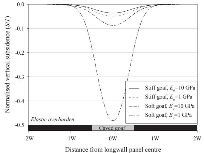
Fig. 4. Subsidence normalised by extracted seam height for an elastic overburden material with varying Young's modulus of the strata ( $E_o$ ) and goaf material – Goaf Model.
