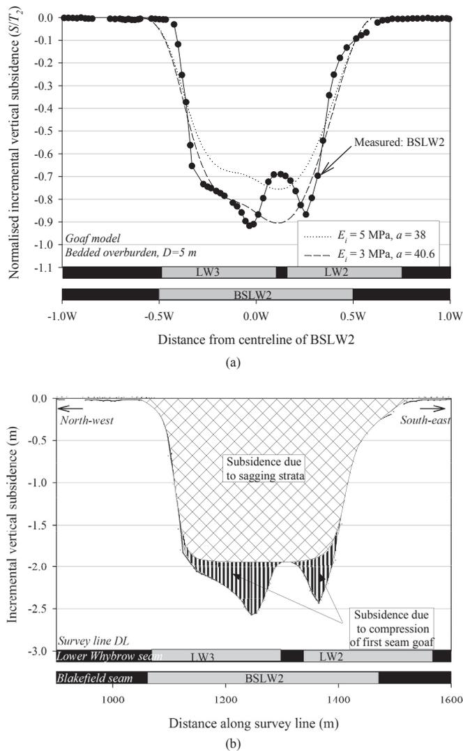
**Fig. 13.** (a) Normalised incremental subsidence for BSLW2 predicted using the Goaf Model with a bedded overburden and the normalised measured subsidence for BSLW2 along DL survey line (values of  $E_i$  and  $a$  identified in the legend correspond to the second seam); (b) Inferred subsurface deformations contributing to the subsidence recorded at the ground surface.
