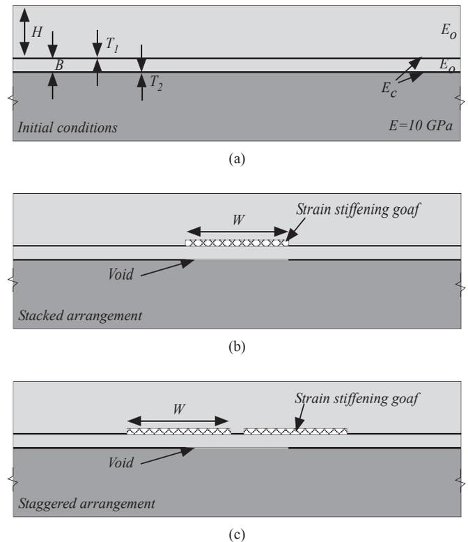
Fig. 9. Schematic drawing of geometry and material properties of (a) initial conditions of both stacked and staggered arrangements, (b) final conditions for the stacked arrangement, and (c) final conditions for the staggered arrangement. As a scale drawing, the void in the second seam is placed as marked but cannot be seen in the figure.
