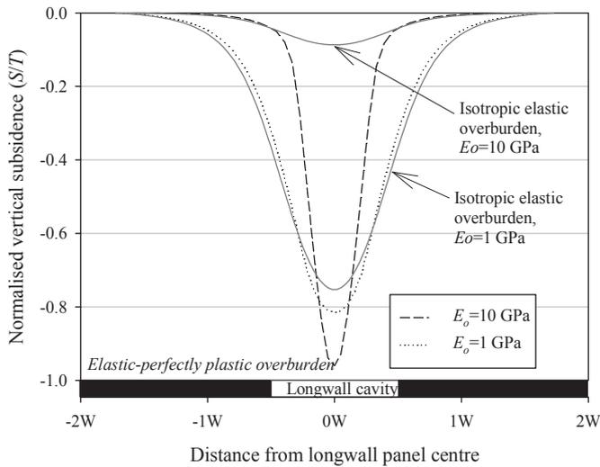
Fig. 5. Normalised surface subsidence for an elastic-perfectly plastic overburden with varying Young's modulus – Cavity Model. Isotropic linear elastic overburden results have been included for comparison.
